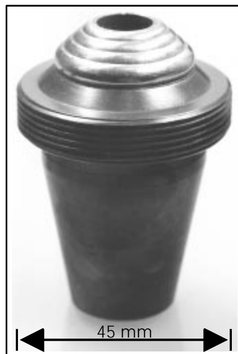
Fig. 8 Nozzle of a spray die-casting machine made of hot work tool steel (1.2343) coated with a cobalt-base alloy (Stellite 157)
